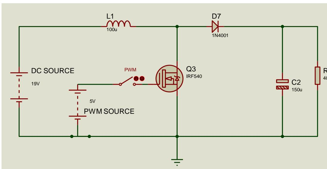
Figure 2.0: DC boost converter Circuit.
