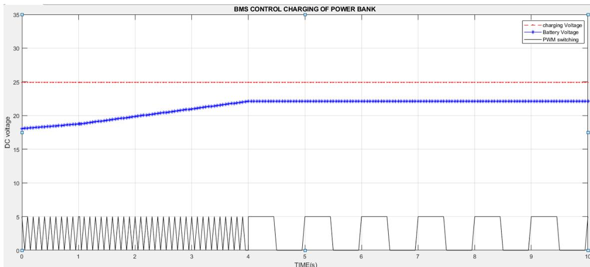
**Figure 5.0:** BMS control charging of power bank.
