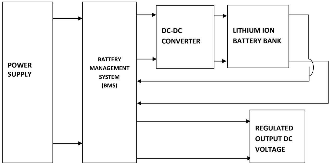
Figure 1.0: Block diagram of a laptop power bank
