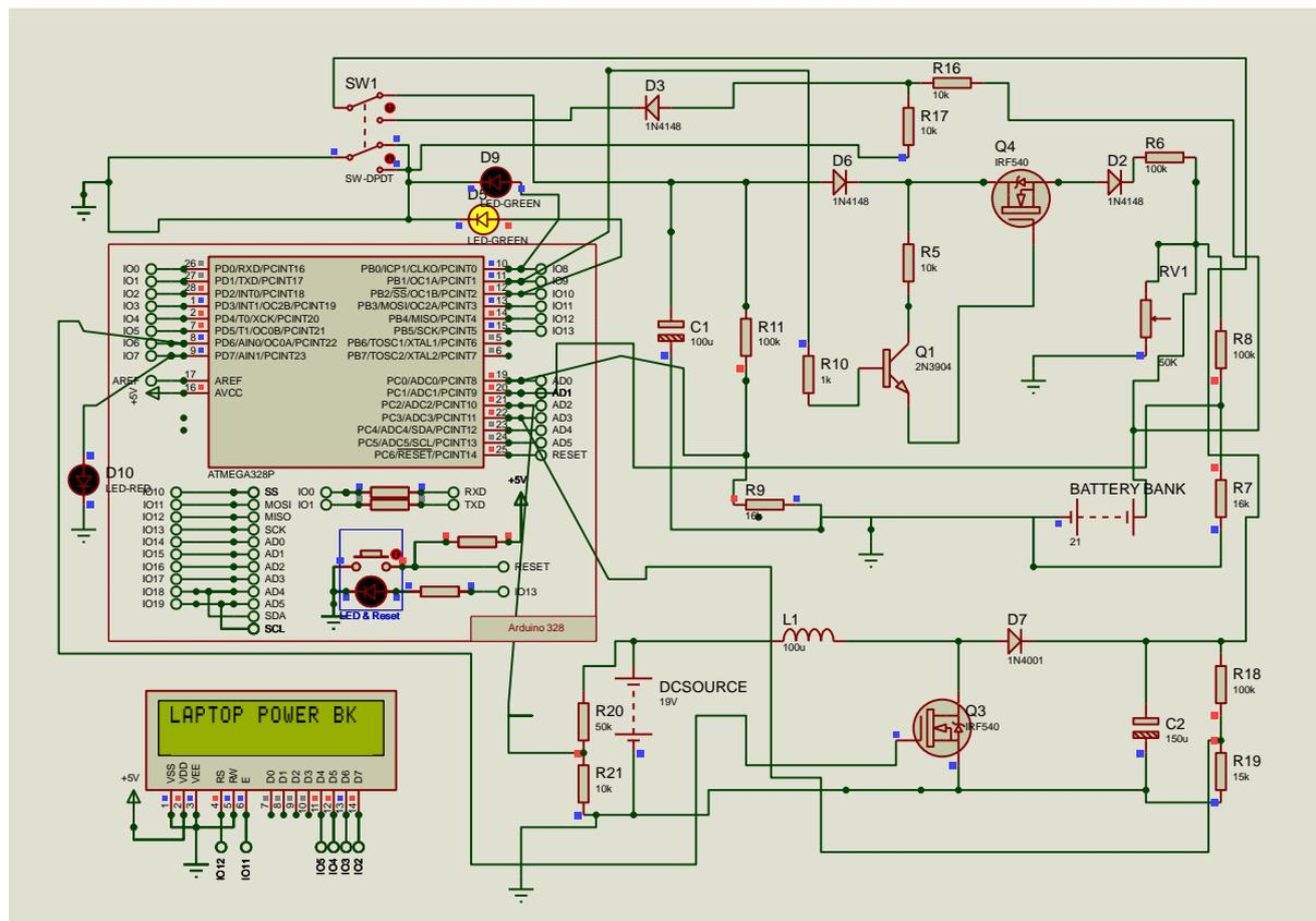
Figure 3.0: Circuit design of a laptop power bank
